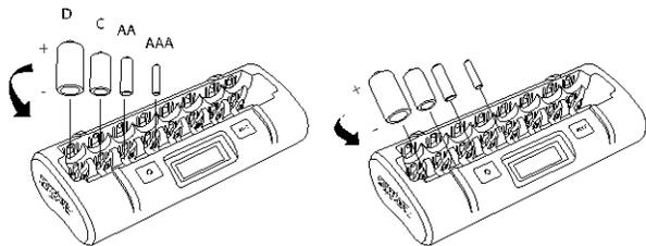
**NOTE:** Ensure that the batteries are **pressed down all the way** to ensure optimal contact.
